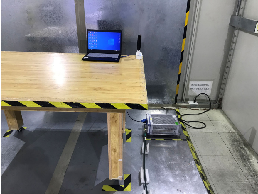
Conducted Emissions (Left View)
