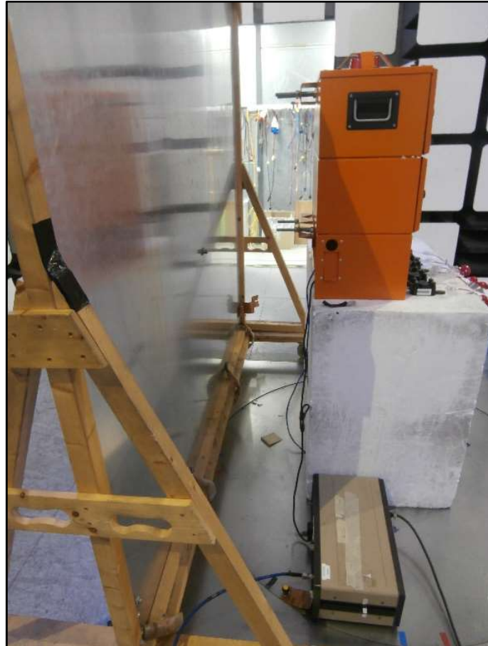
Figure 11 – Conducted Disturbance at Mains Terminals
