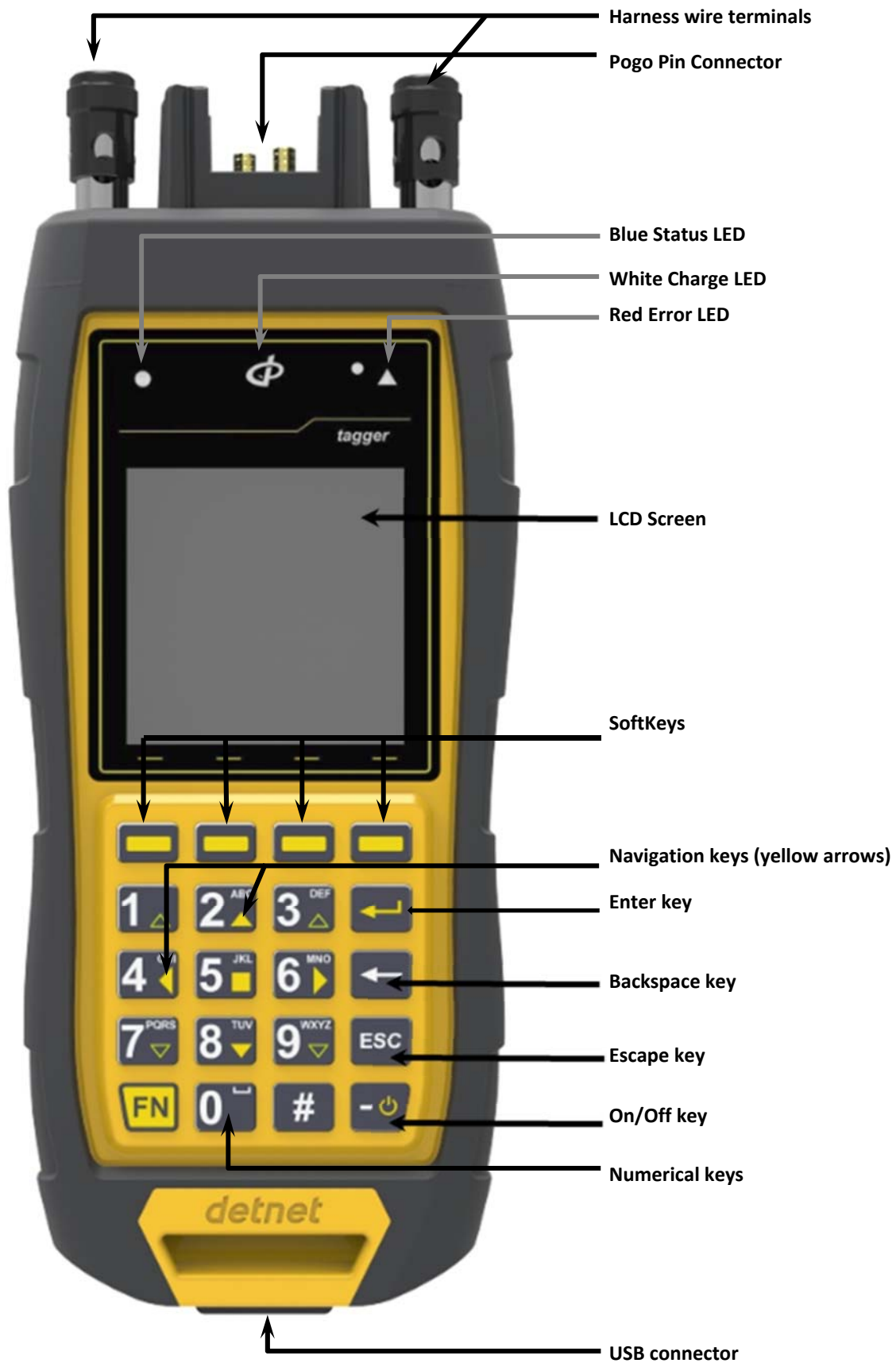
Figure 5: CE4 Tagger Component Identification
