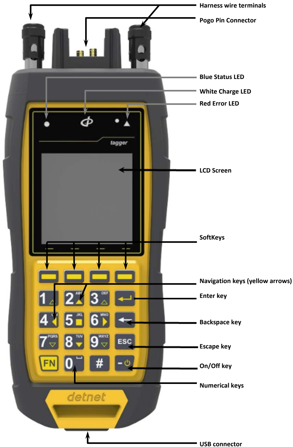
Figure 5: CE4 Tagger Component Identification
