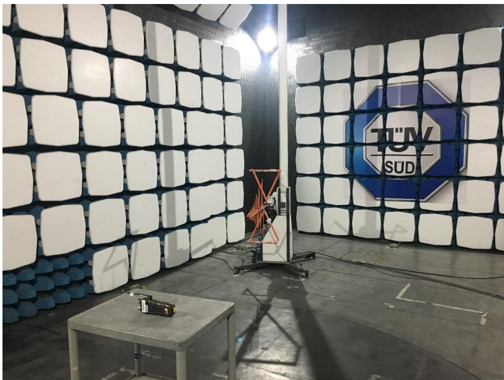
Figure 30 – Test Setup- 30 MHz to 1 GHz, Y Orientation
