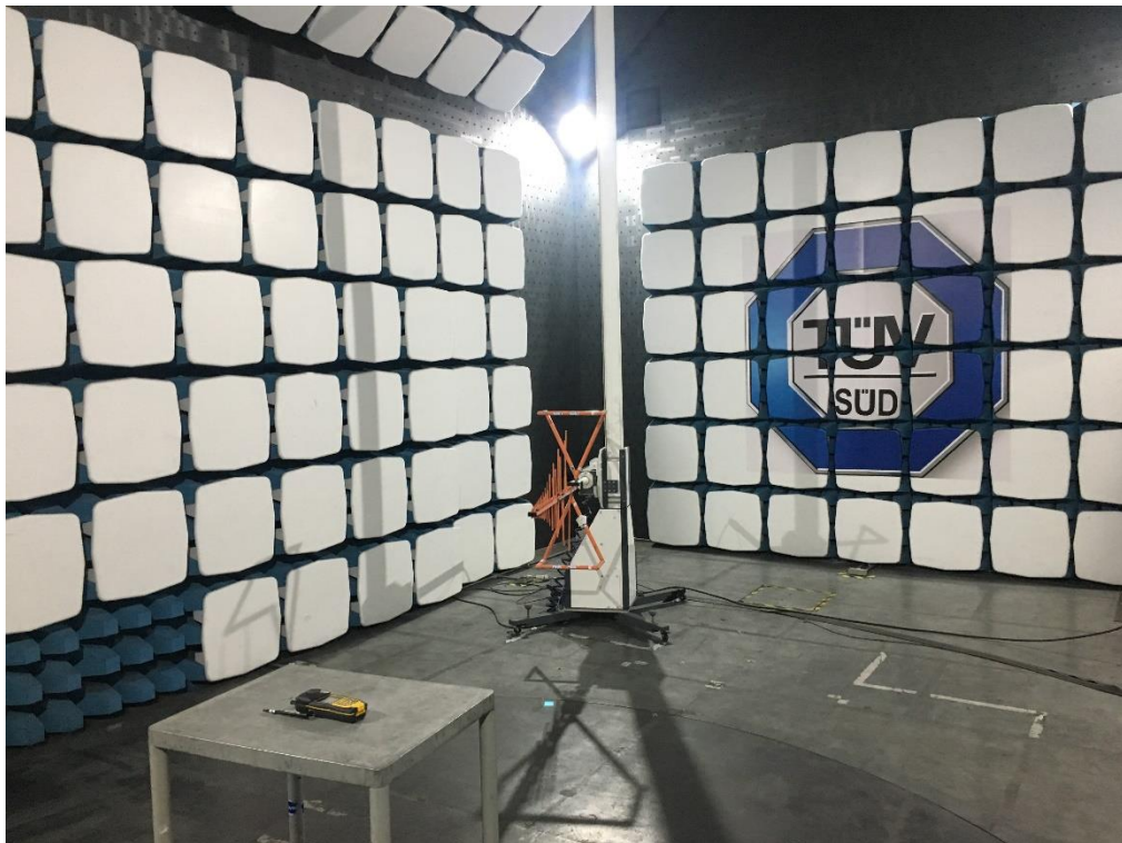
Figure 29 – Test Setup- 30 MHz to 1 GHz, X Orientation
