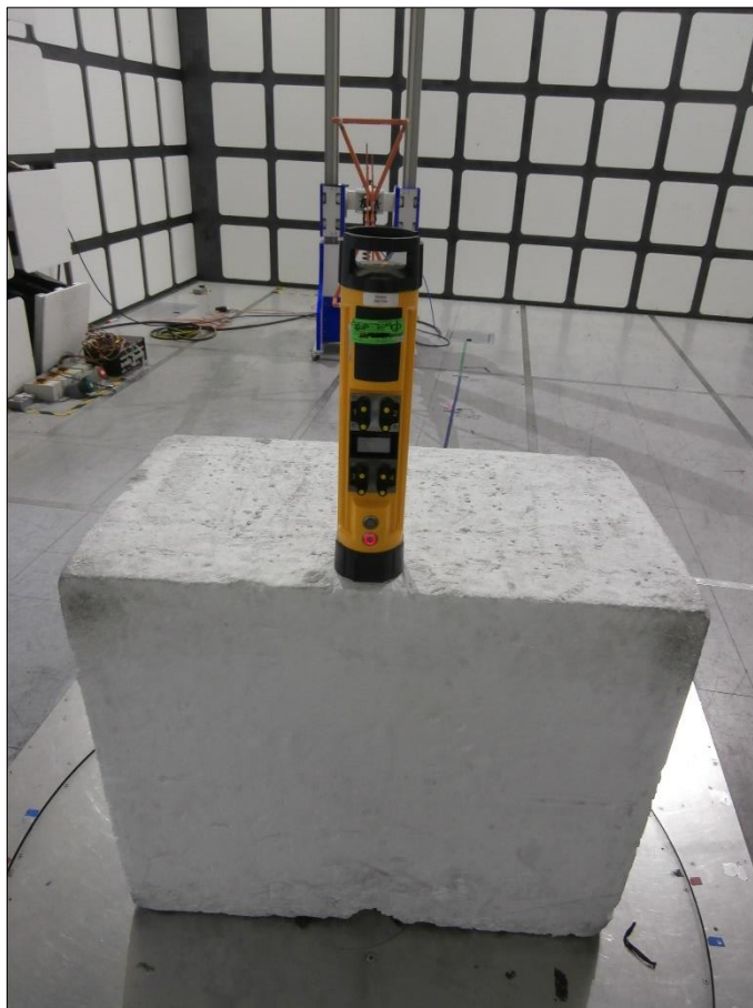
Figure 20 - Test Setup - 30 MHz to 1 GHz
