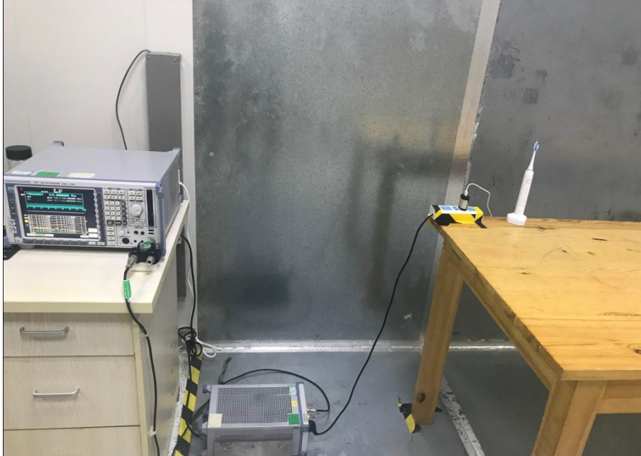
Radiated Spurious Emissions Test Frequency From 9kHz-30MHz
