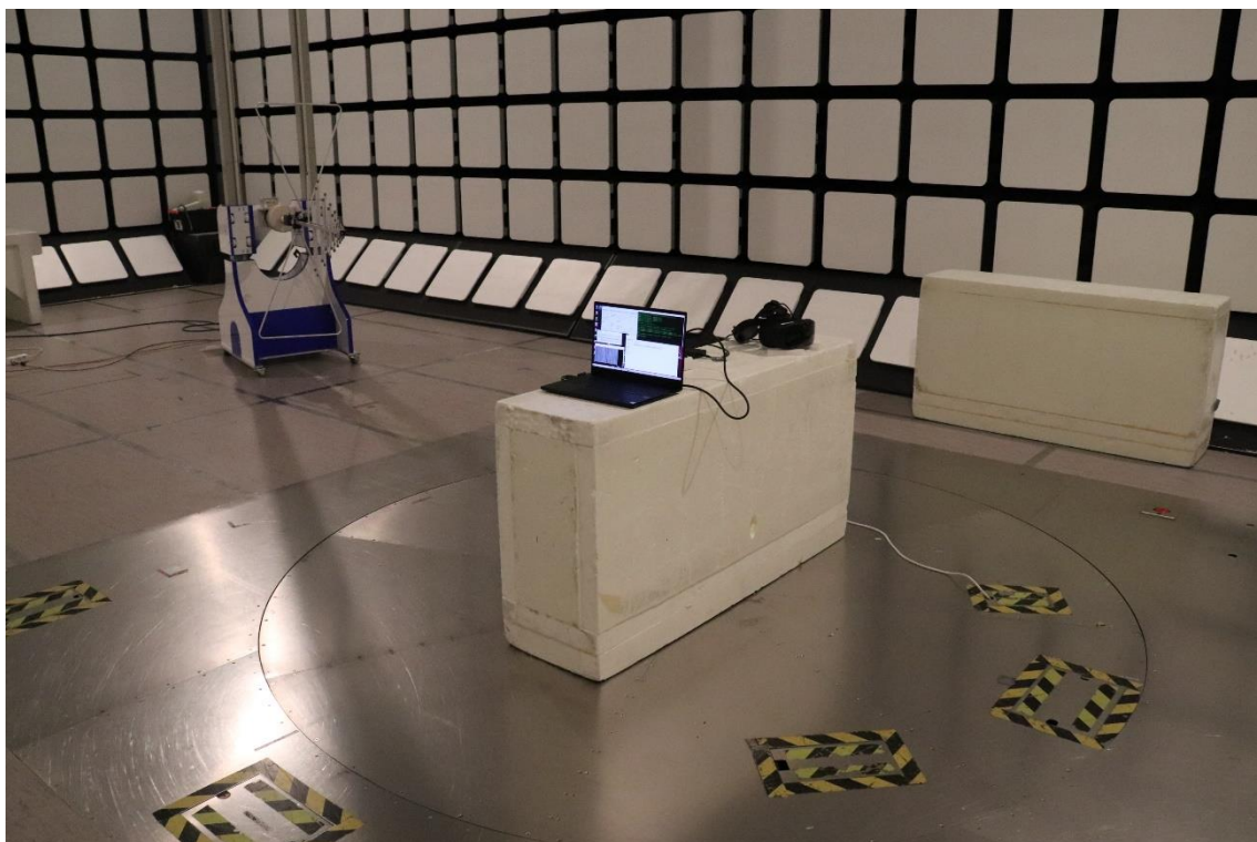
Photograph 3. Test setup for Radiated Emissions (30 – 1000 MHz)
