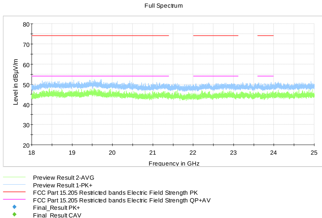
Figure 20: Unwanted emissions 18 – 25 GHz (ch. config. 3)
