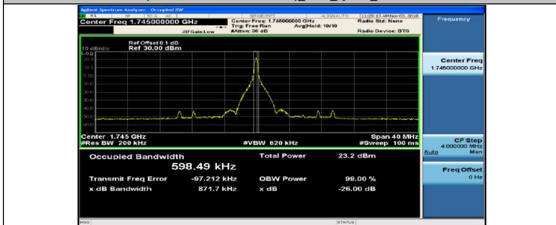
(Channel Bandwidth:20 MHz)_HCH_QPSK_1RB#99
