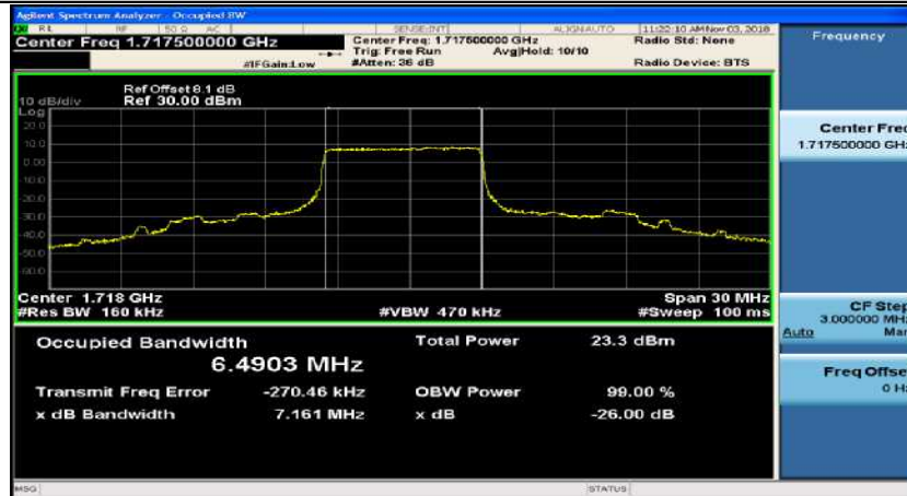
(Channel Bandwidth:15 MHz)_LCH_QPSK_37RB#38
