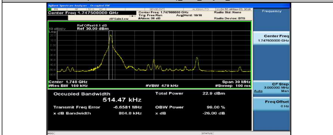
(Channel Bandwidth:15 MHz)_HCH_16QAM_1RB#37
