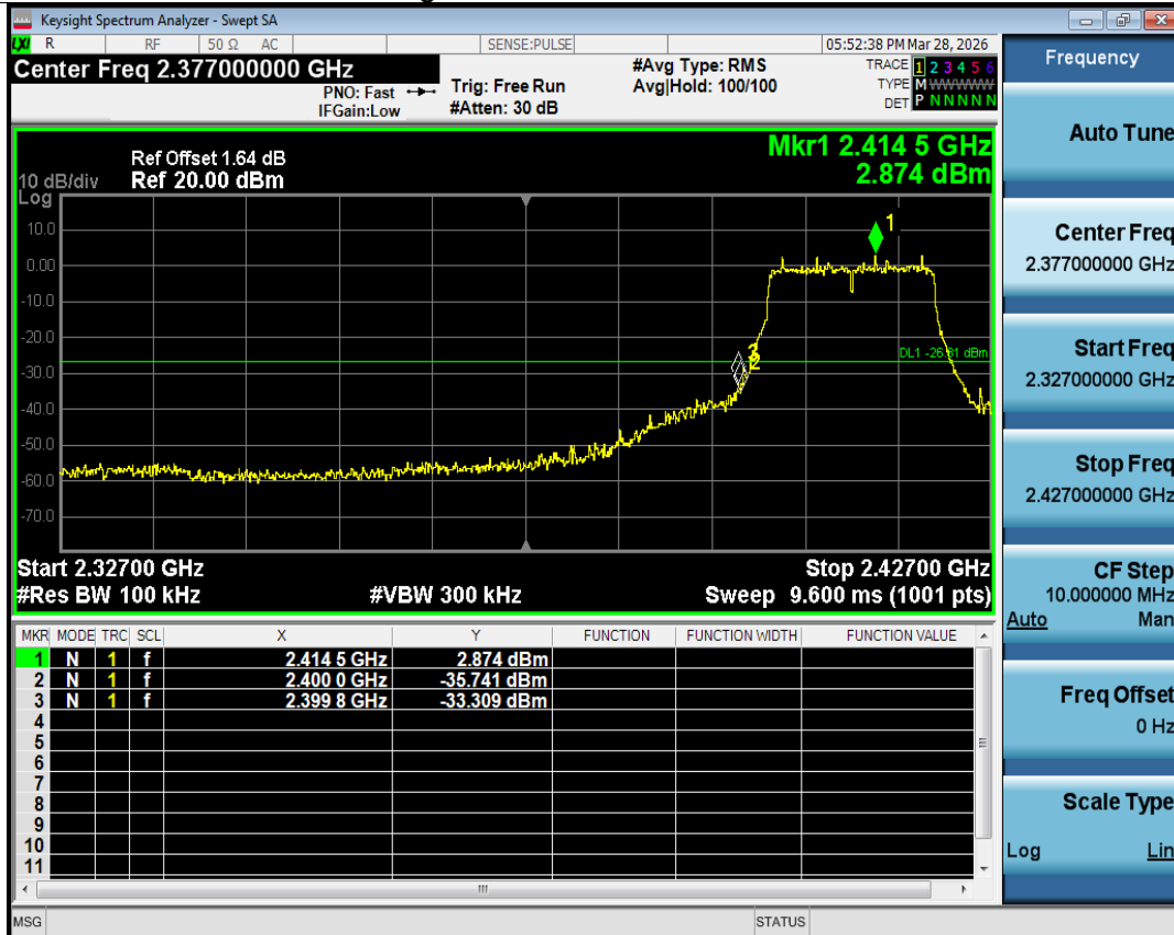
Band Edge NVNT n20 2412MHz Ant1 Emission
