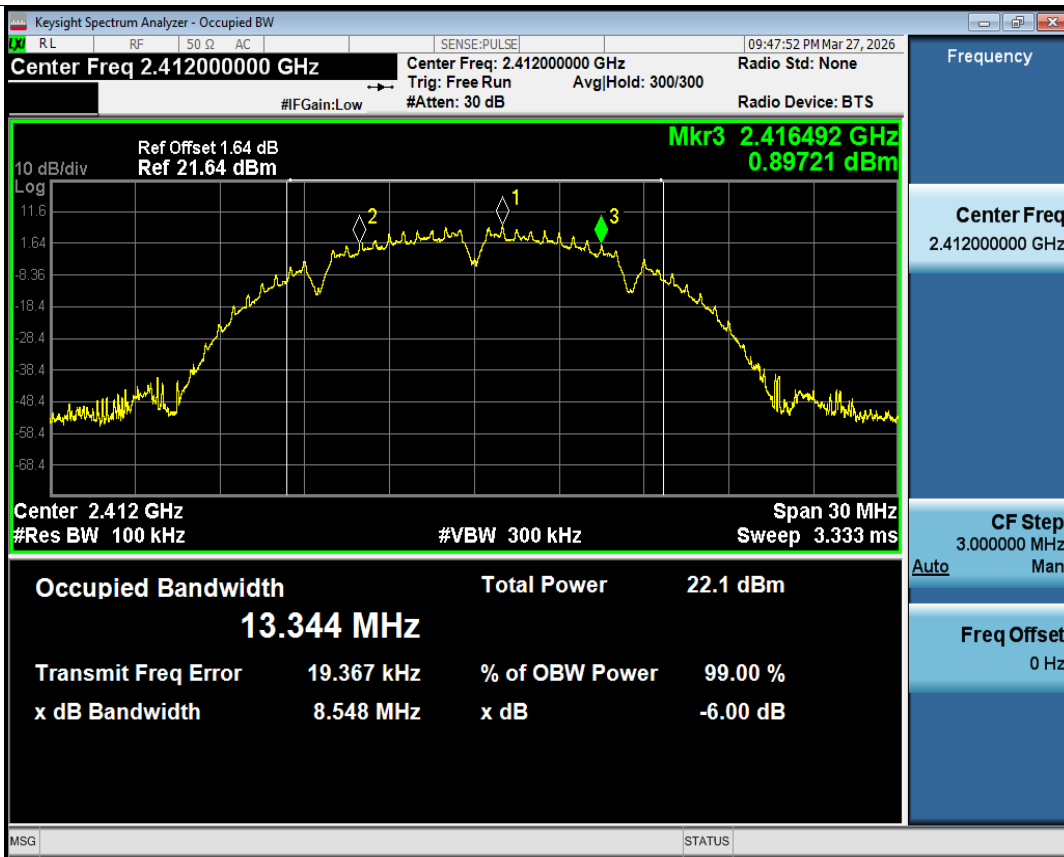
-6dB Bandwidth NVNT b 2412MHz Ant1
