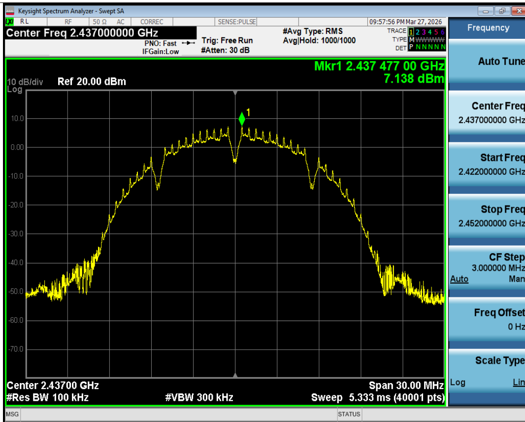
Tx. Spurious NVNT b 2437MHz Ant1 Ref
