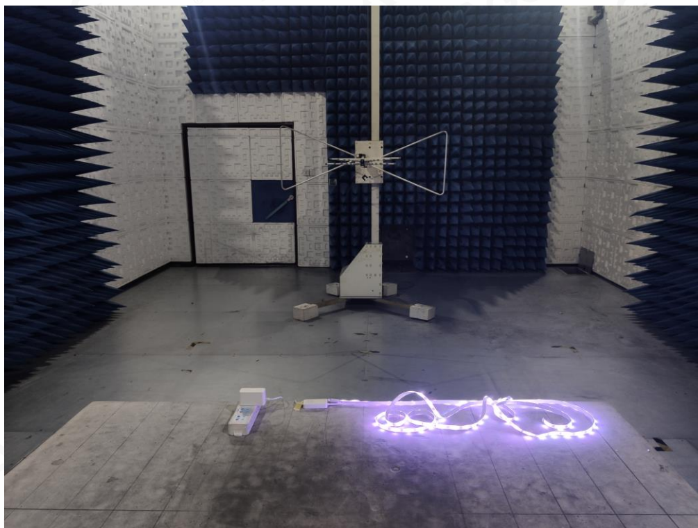
FCC RADIATED EMISSION TEST SETUP ABOVE 1GHZ
