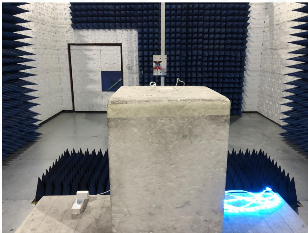
FCC RADIATED EMISSION TEST SETUP ABOVE 1GHZ
