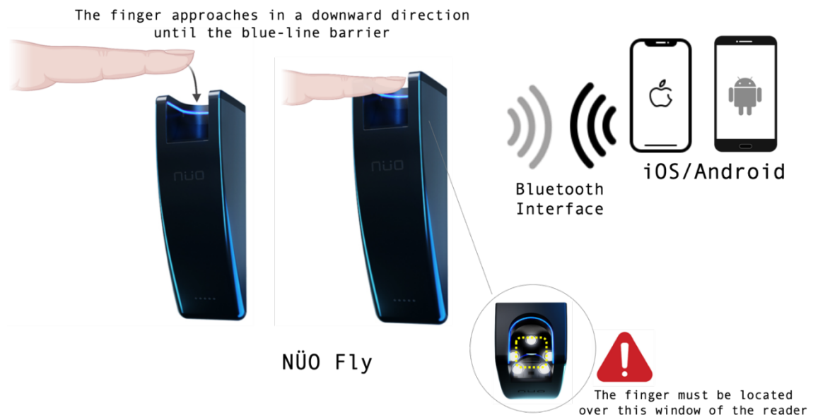
Figure 4. Operational description of NÜO FLY1 reader.
