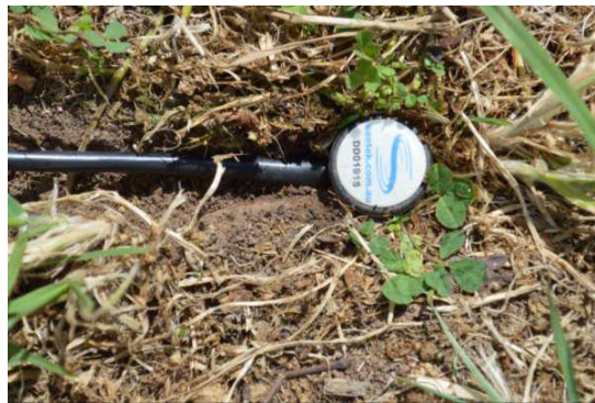
Figure 4 Properly installed probe
