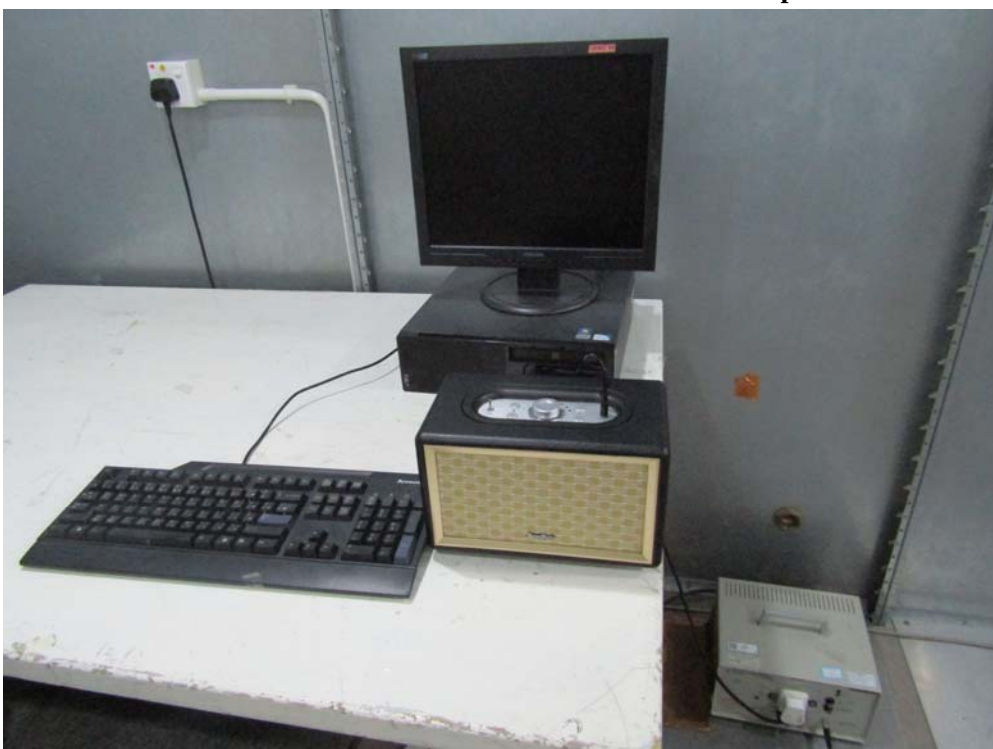
Measurement of Conducted Emission Test Set Up
