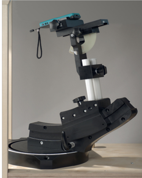
F-2. Device Holder for Transmitters
