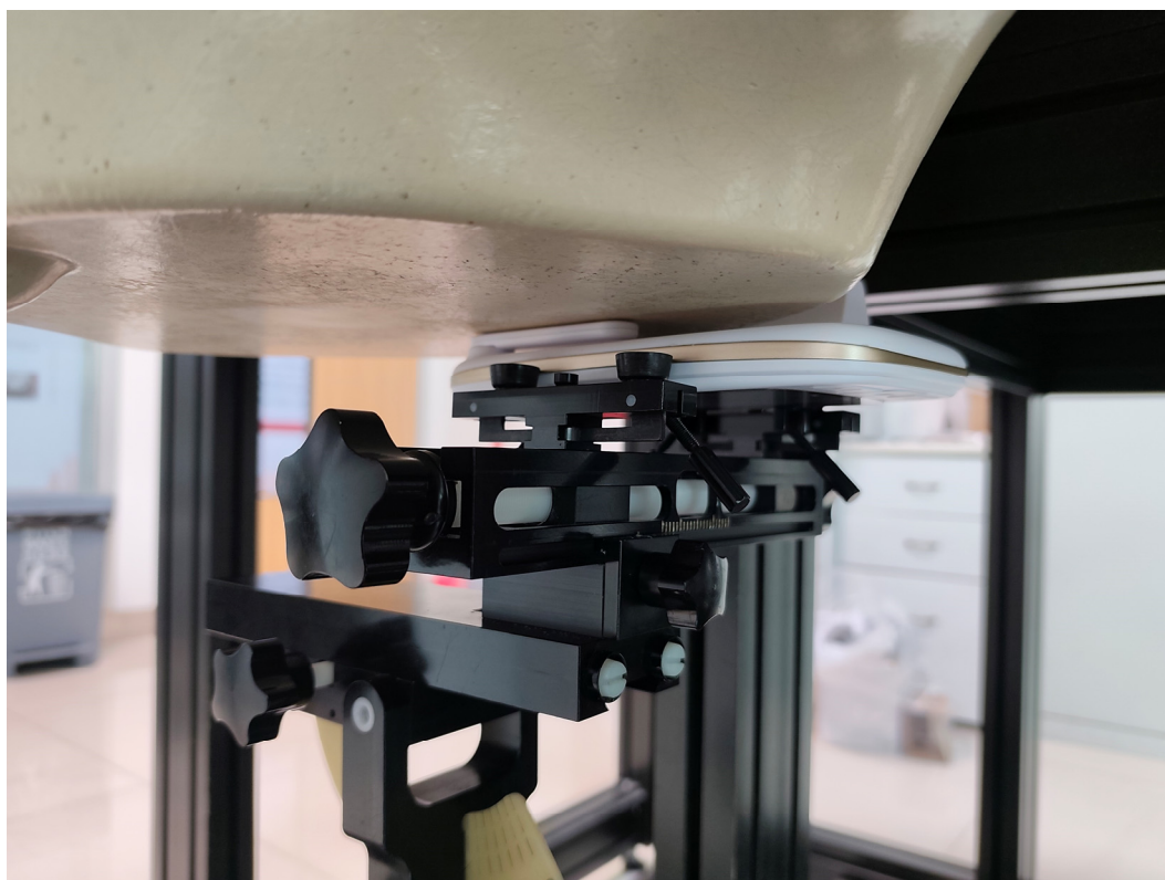
Body Back Close Setup Photo (0 mm)
