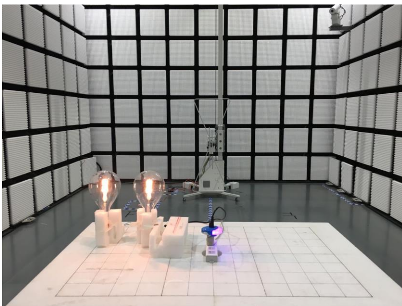
Fig.4 Radiated emission setup photo(30MHz-1GHz)
