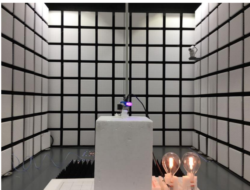
Fig.6 Radiated emission setup photo(Above 1GHz)
