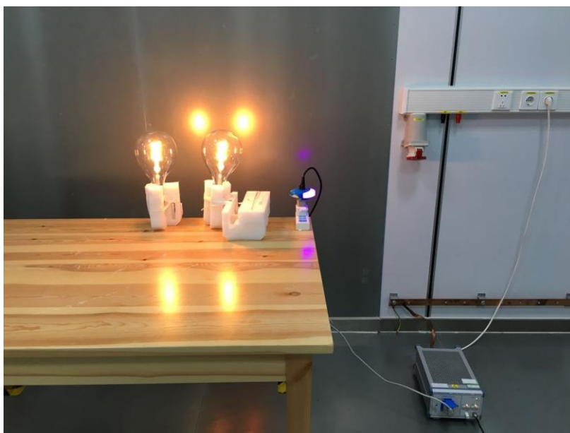
Fig.7 Power line conducted emission setup photo
