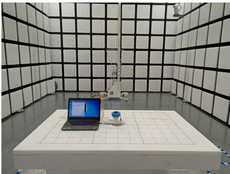
Fig.3 Radiated emission setup photo(30MHz-1GHz)
