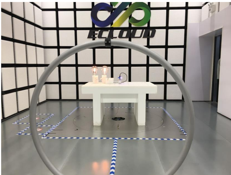
Fig.2 Radiated emission setup photo(Below 30MHz)
