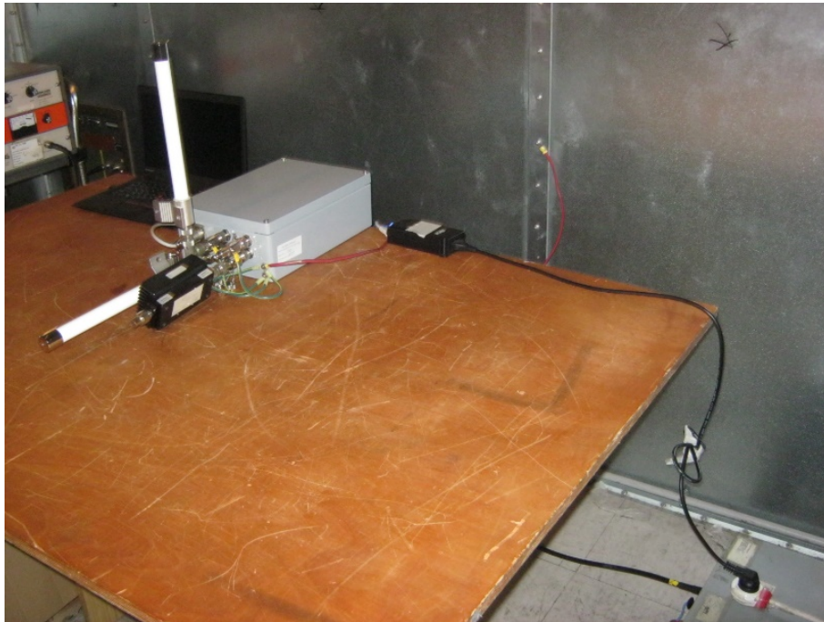
Figure 3. Conducted Emission from AC Mains Line Test
