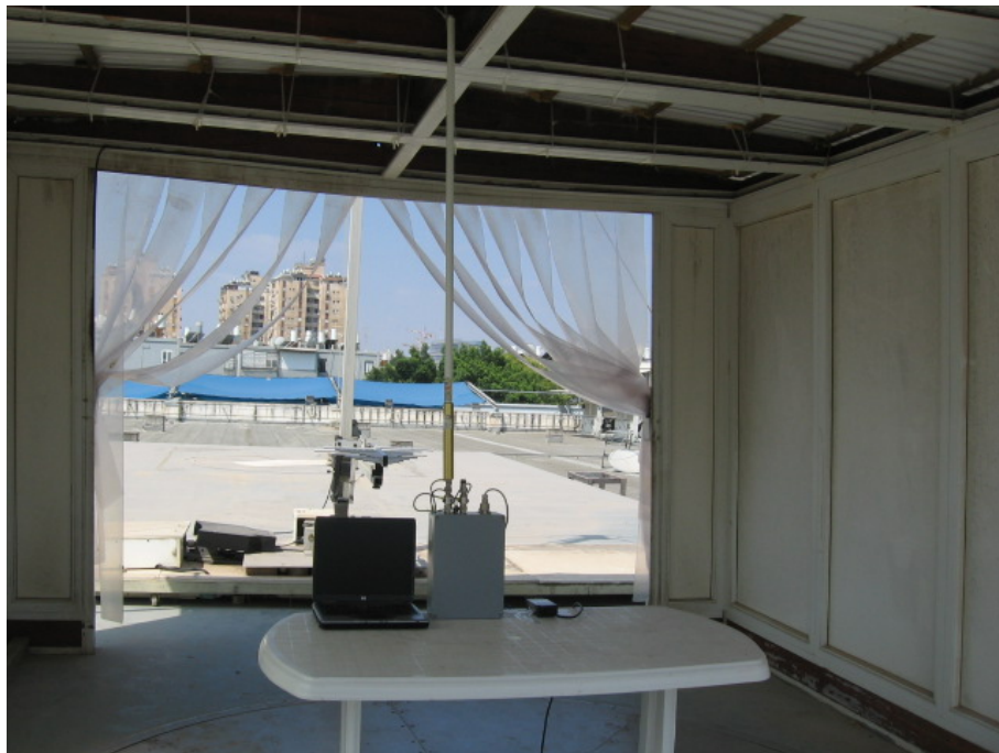
Figure 7. Radiated Emission Test, 200-1000MHz
