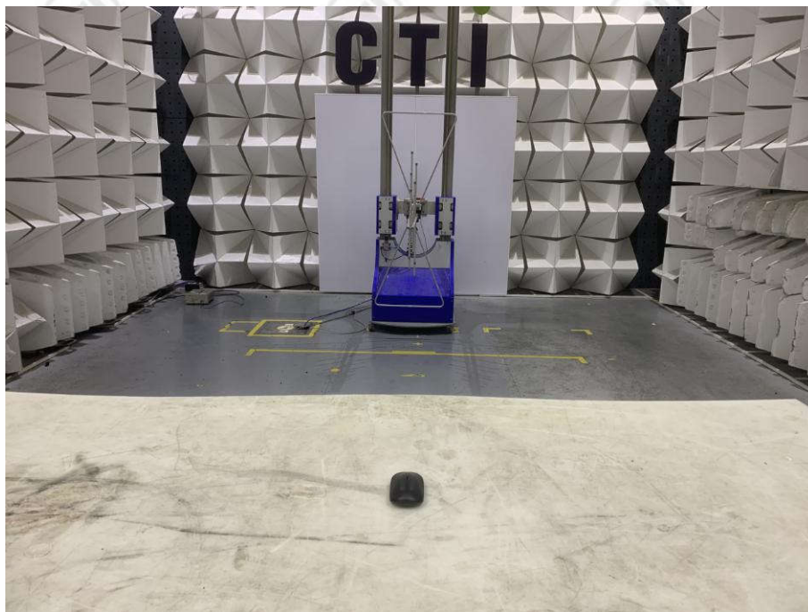
Radiated spurious emission Test Setup-1(Below 1GHz)
