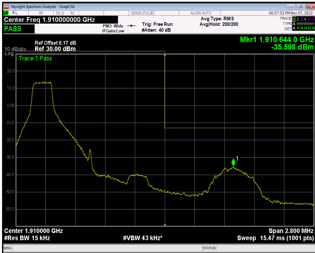
Band2 QPSK BW=1.4MHz Channel=19193 RB Size=1 Position=#Max
