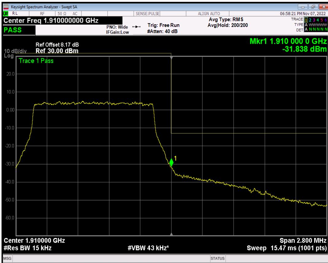
Band2 QPSK BW=3MHz Channel=18615 RB Size=1 Position=#0
