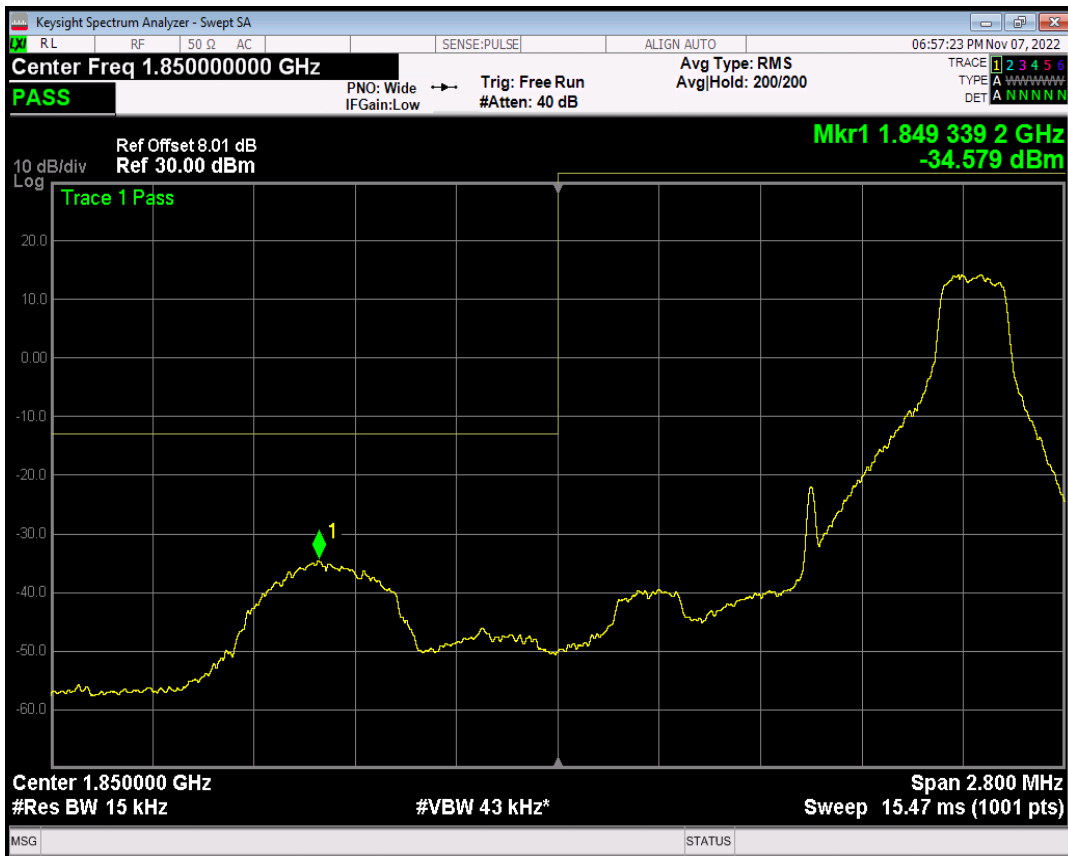
Band2 QPSK BW=1.4MHz Channel=18607 RB Size=6 Position=#0
