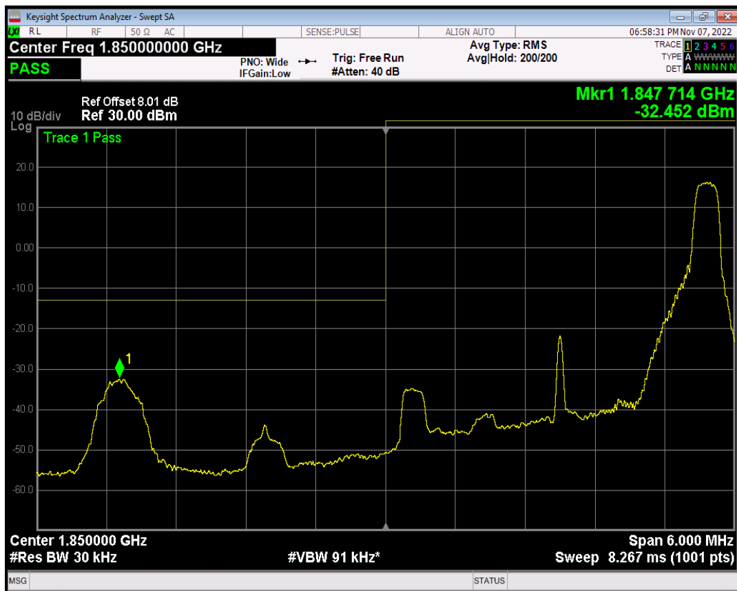
Band2 QPSK BW=3MHz Channel=18615 RB Size=15 Position=#0
