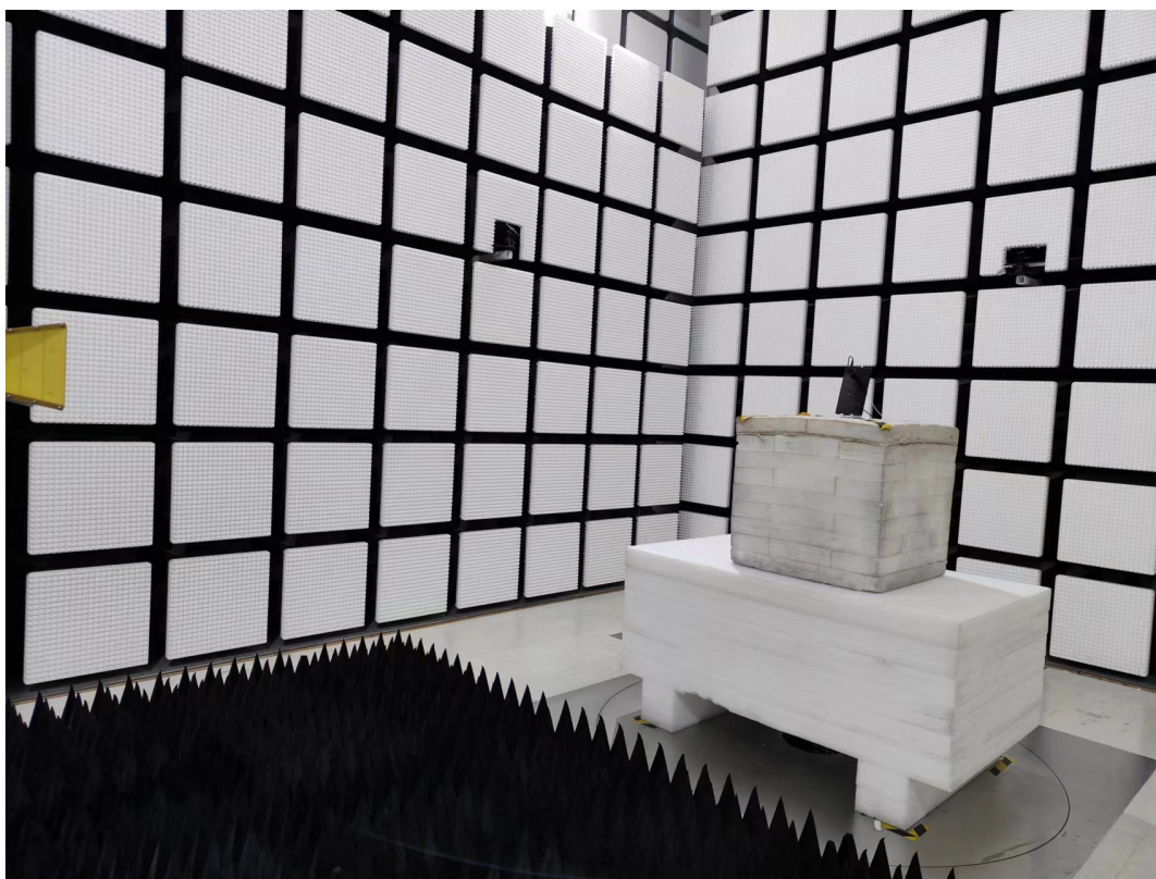
Radiated Emission Above 1GHz View
