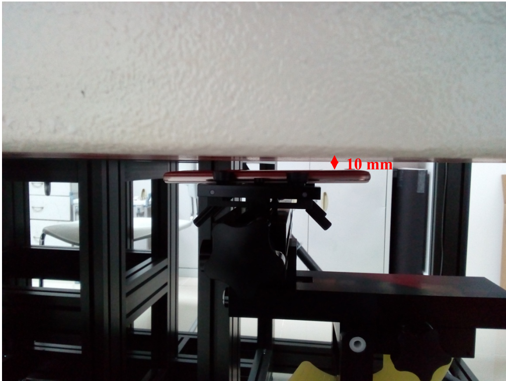
Body (Worn) Back Setup Photo (10mm)
