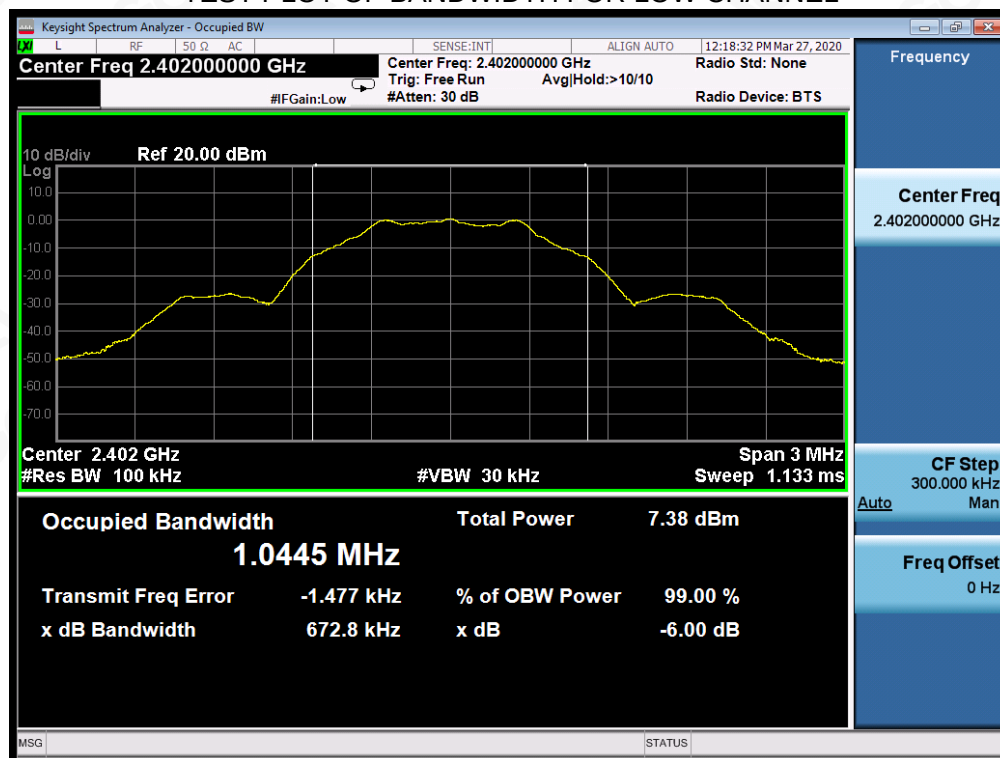
TEST PLOT OF BANDWIDTH FOR LOW CHANNEL
