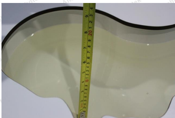
Liquid depth in the head phantom (2600MHz)
