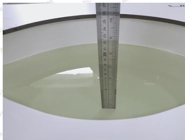
Liquid depth in the body phantom (2450MHz)
