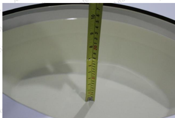
Liquid depth in the body phantom (2600MHz)
