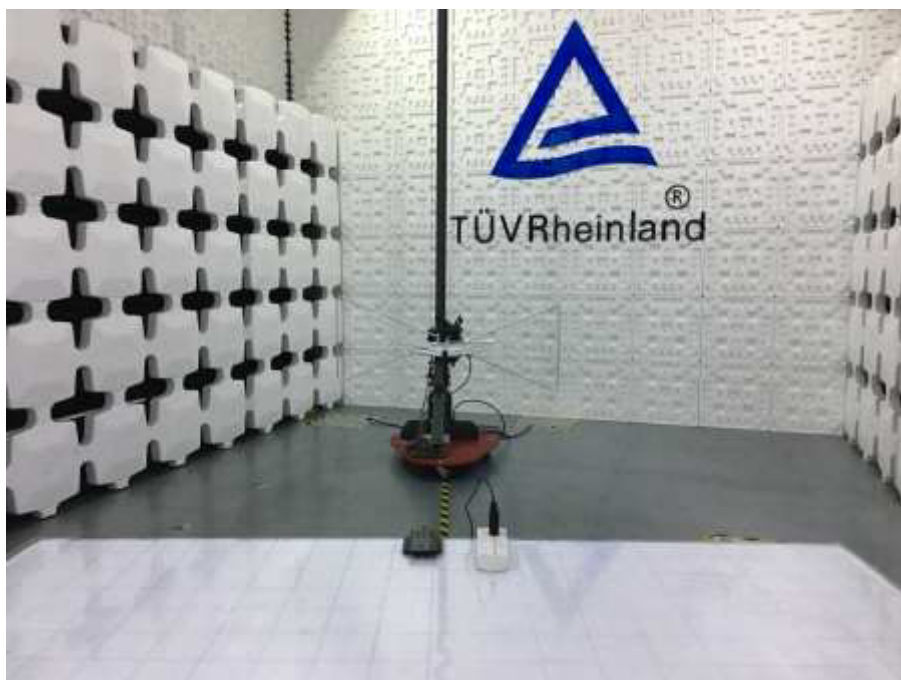
Photograph 2: Set-up photo for Radiated Emission, 30MHz - 1GHz
