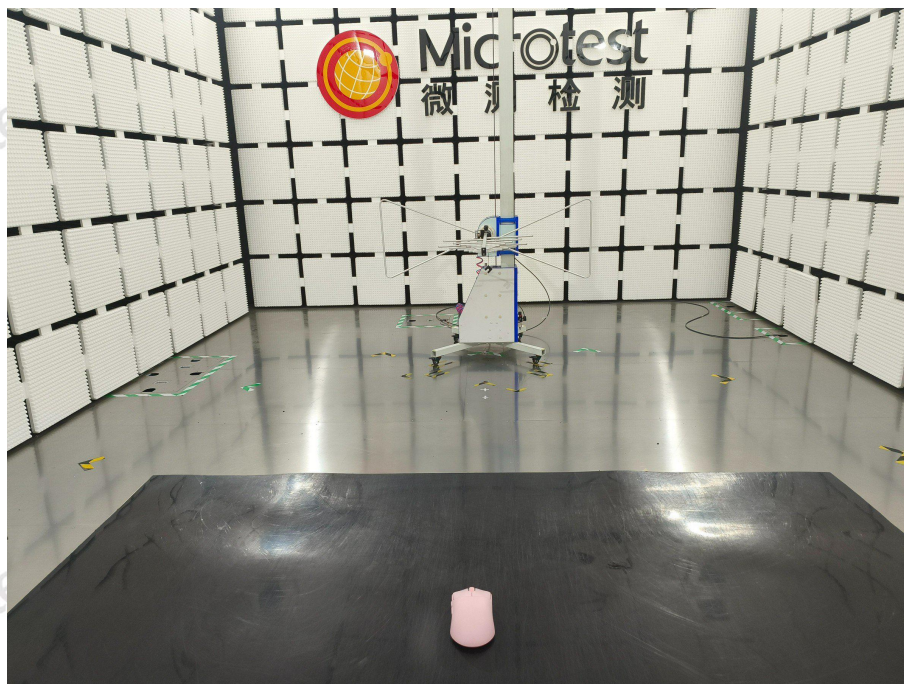
Radiated emissions (below 1GHz)
