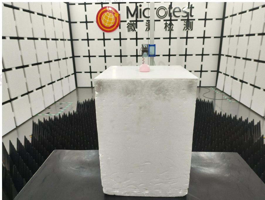
Radiated emissions (above 1GHz)
