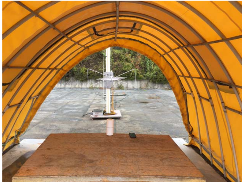
Photograph 2 : Setup for radiated Emissions (above 1 GHz)
