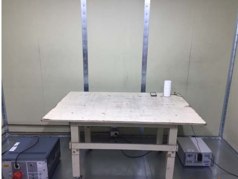
Photograph 3 : Setup for Conducted Emissions
