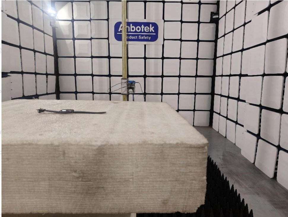
Photo of Radiation Emission Test (above 1GHz)
