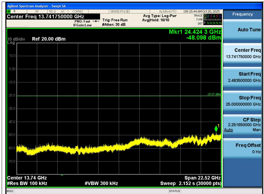
Test_Graph_EDR_ANT1_2441_2Mbps_Higher Band Emissions
