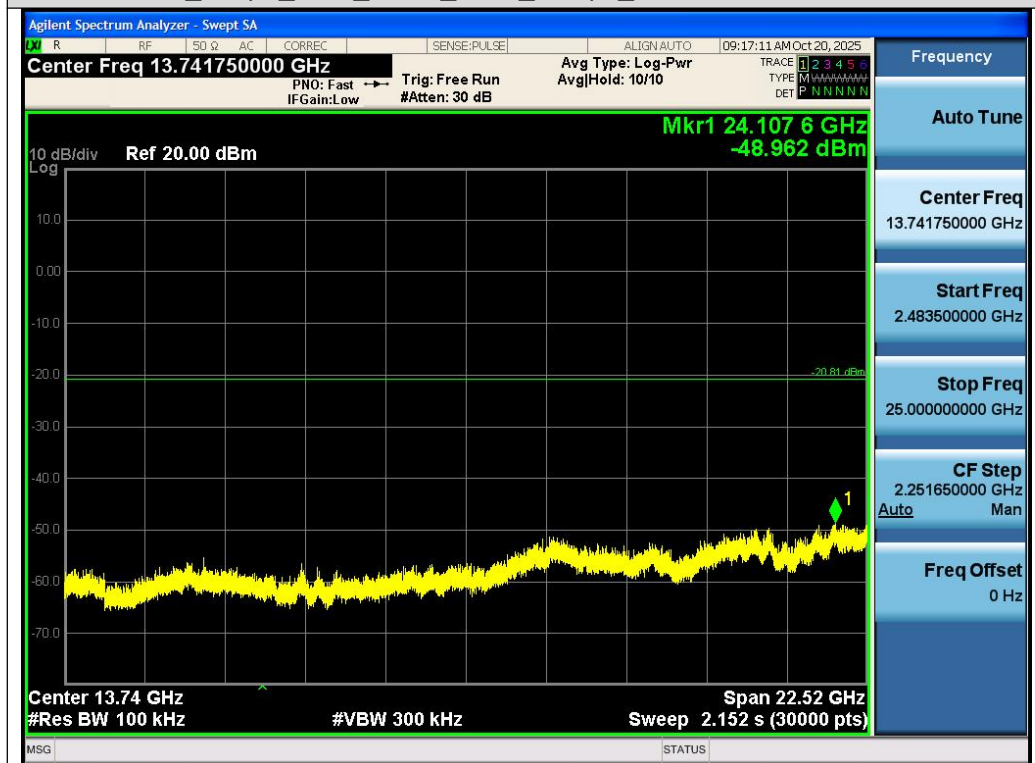
Test_Graph_EDR_ANT1_2402_2Mbps_Higher Band Emissions
