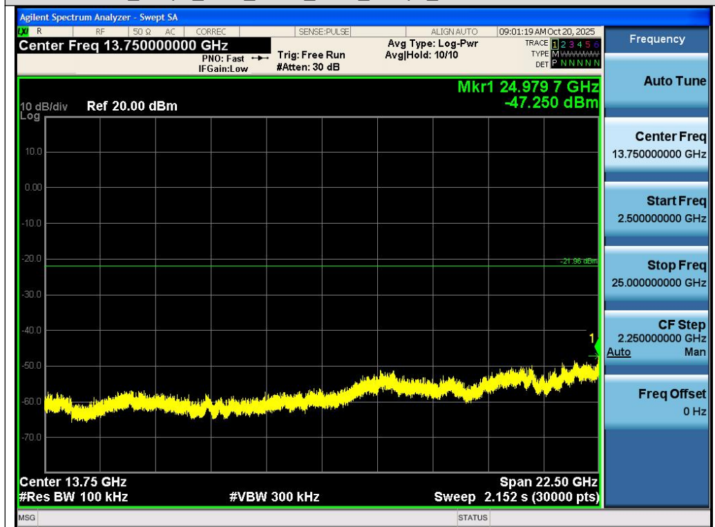
Test_Graph_EDR_ANT1_2480_2Mbps_Higher Band Emissions
