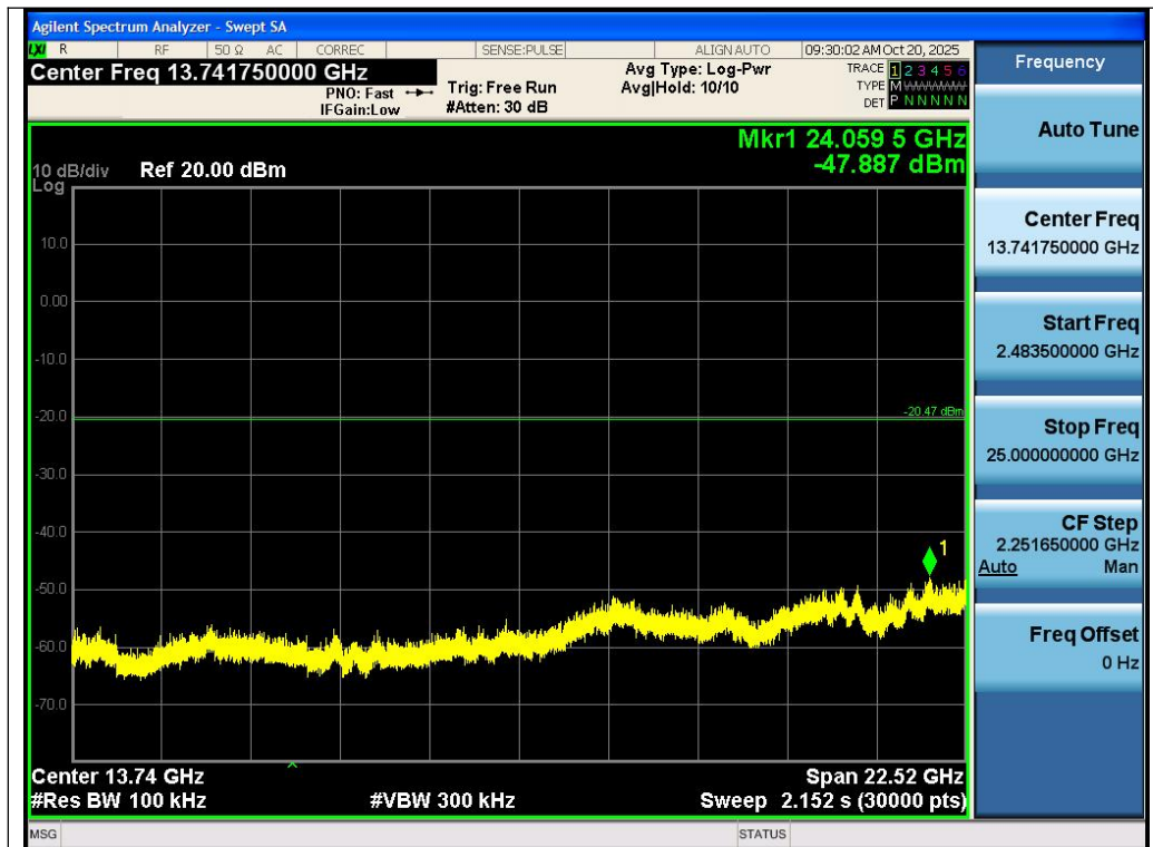
Test_Graph_EDR_ANT1_2402_3Mbps_Higher Band Emissions
