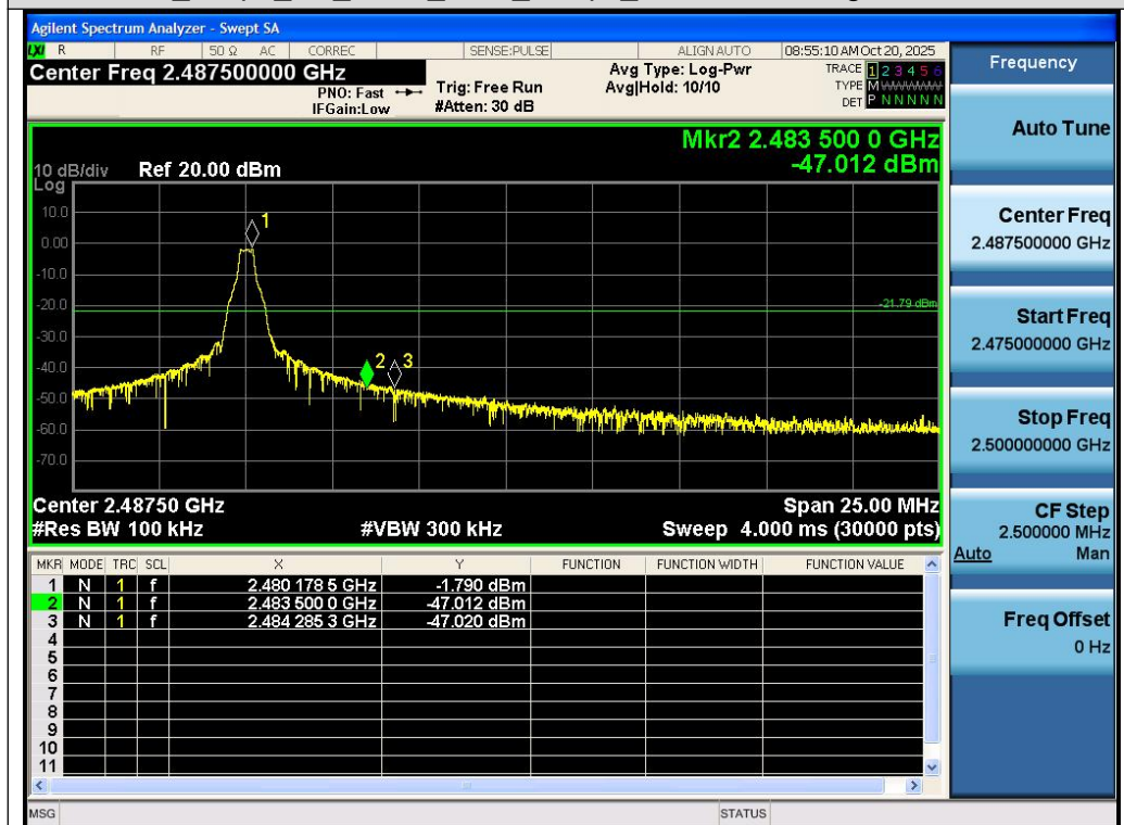
Test_Graph_BR_ANT1_2480_1Mbps_Higher Band Edge Emissions
