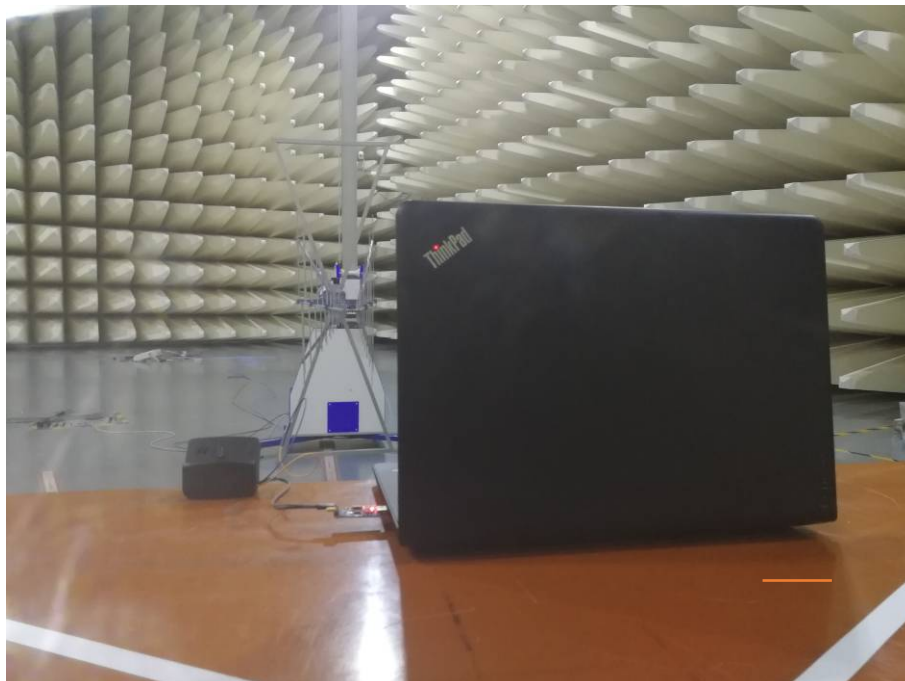
Spurious Radiated Emissions Test setup (below 1GHz)
