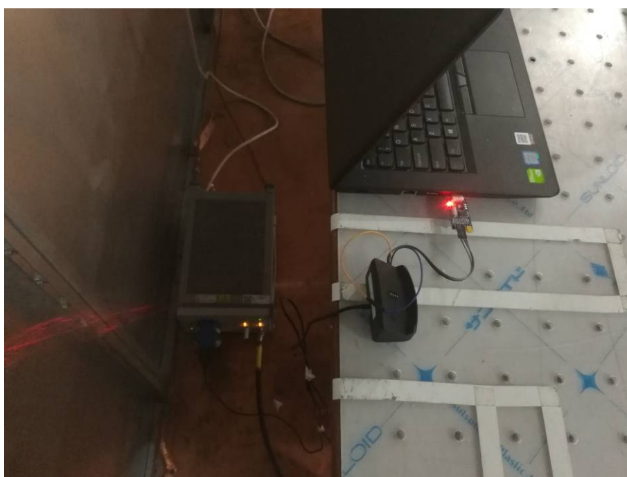
Conducted Emissions Test Setup (with charger)
