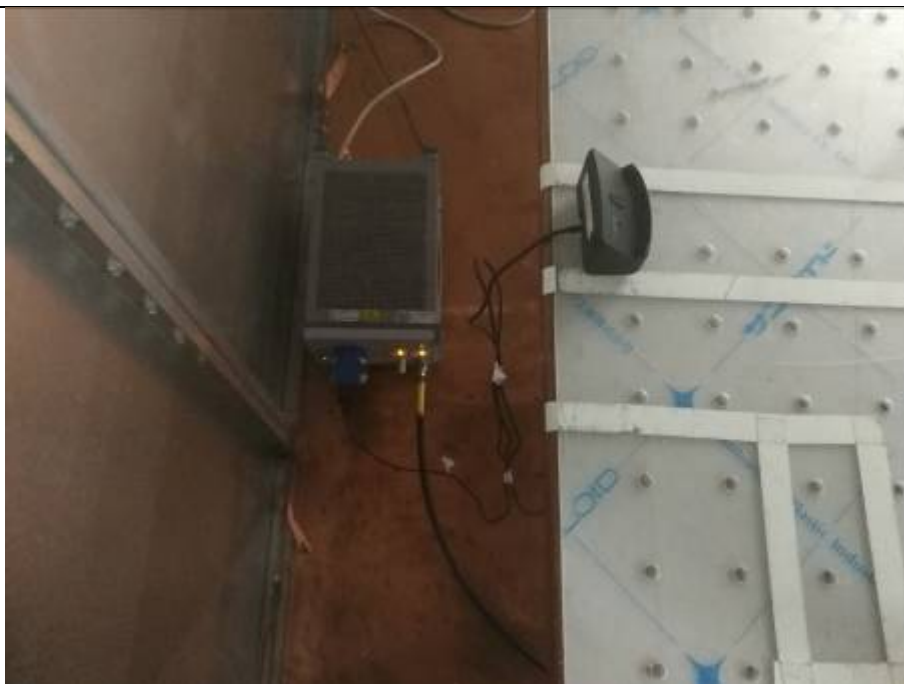
Conducted Emissions Test Setup
