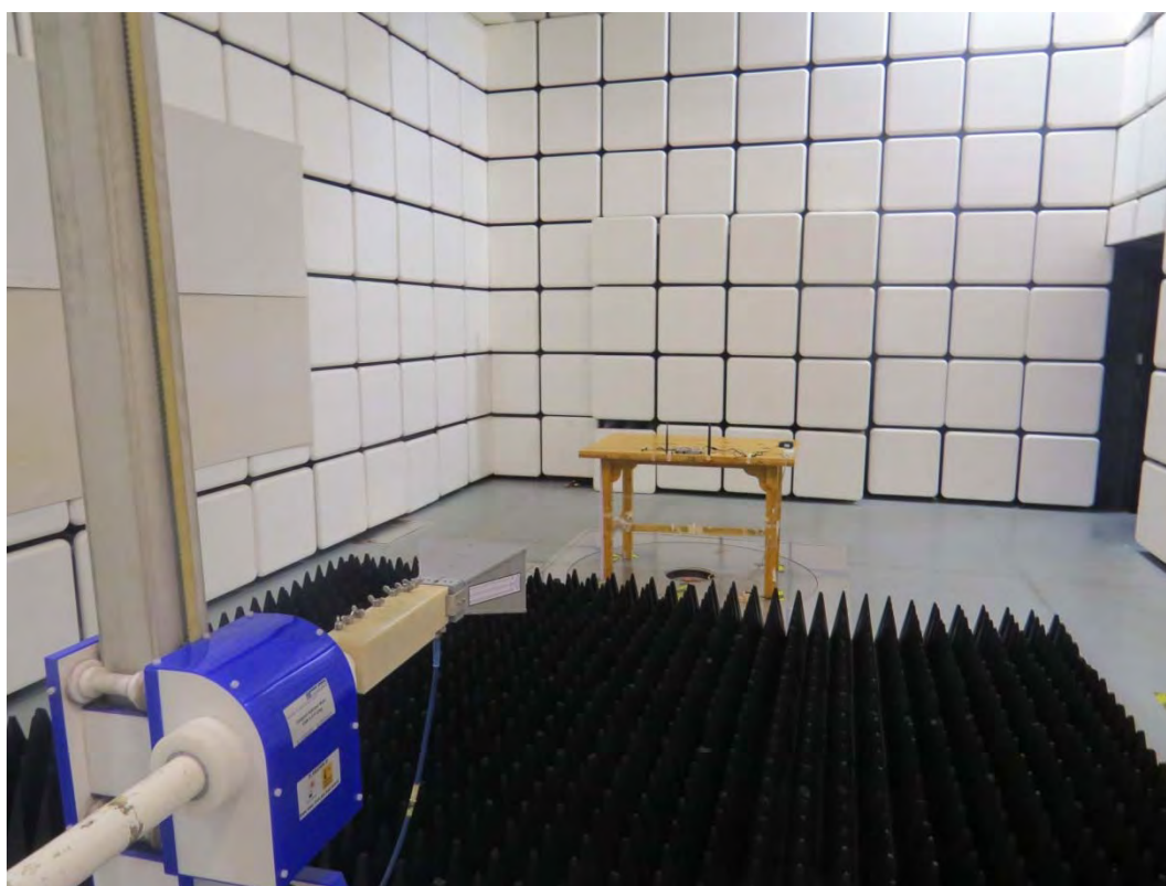
Picture 2: Radiated Spurious Emissions Test setup
