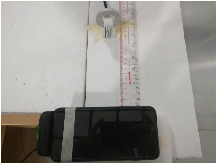
H-field Test Setup Photo Positon B(15mm)
