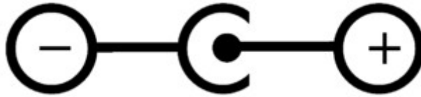
Drawing 1: Power Jack polarity
