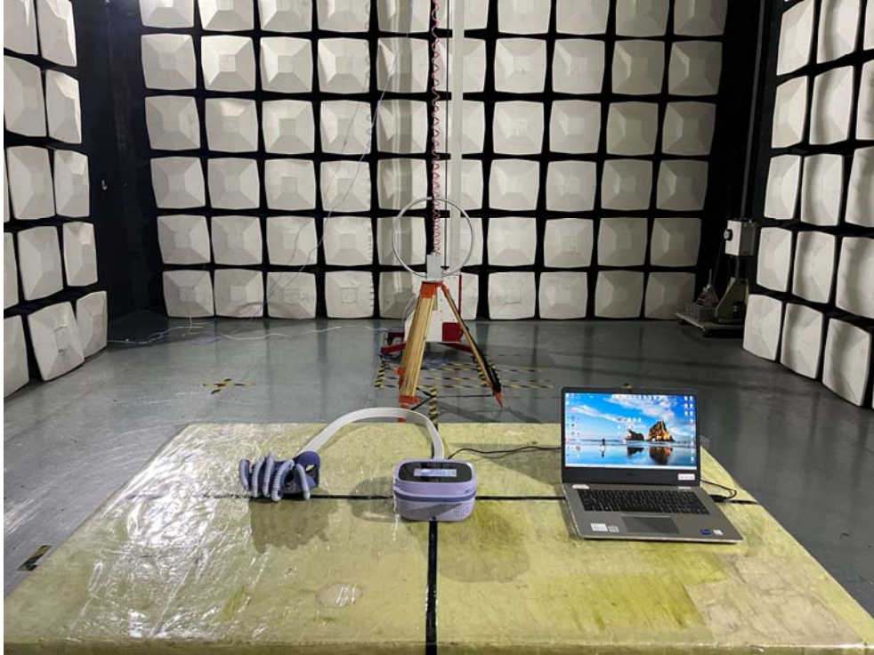
Test Photo Radiated emission (Below 30MHz)
