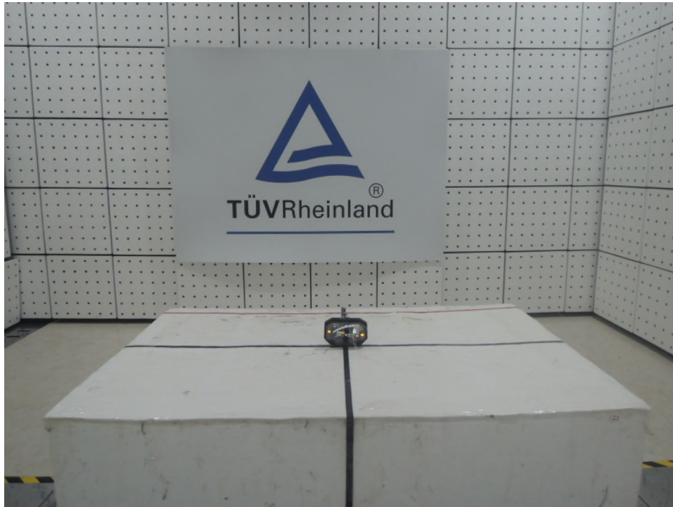
Photograph 9: Set-up for Spurious Emissions (Back View 1) – Model 8198
