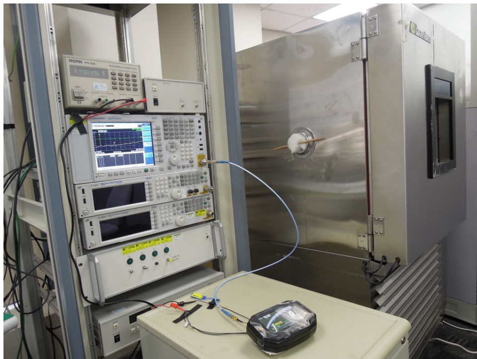
Photograph 13: Set-up for Conducted testing
