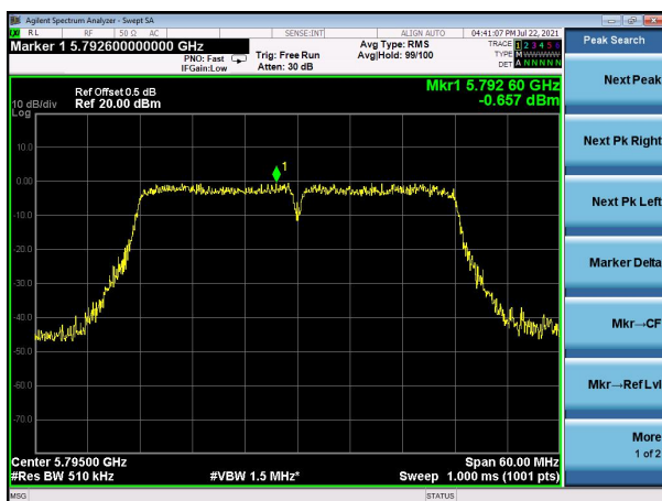
(802.11ac40) PSD plot on channel 159
