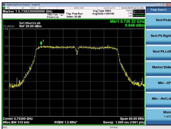
(802.11ac40) PSD plot on channel 151
