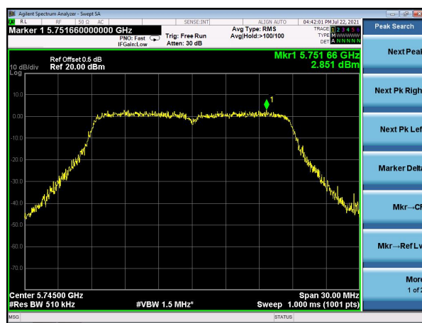
(802.11n20) PSD plot on channel 157
