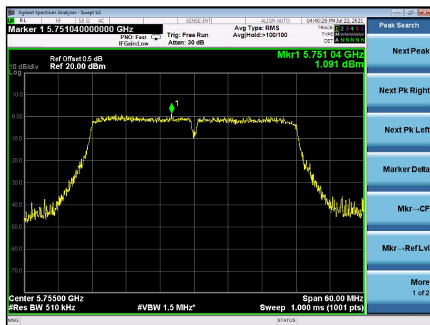
(802.11n40) PSD plot on channel 159
