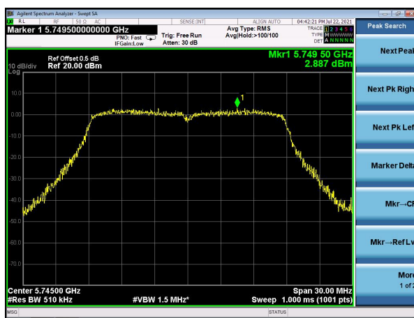
(802.11ac20) PSD plot on channel 157
