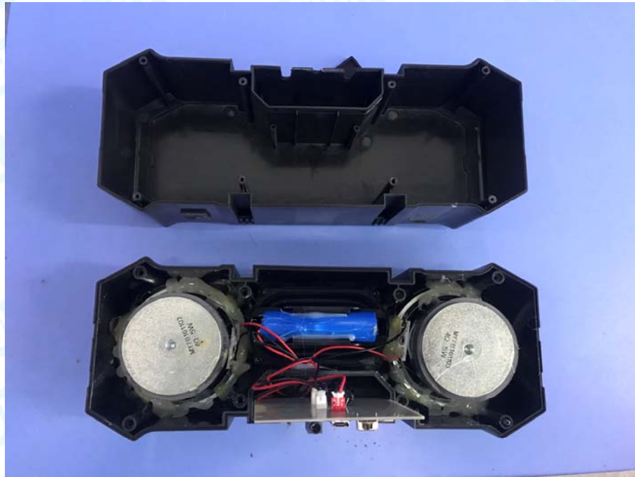
Photo 9 Internal of EUT
