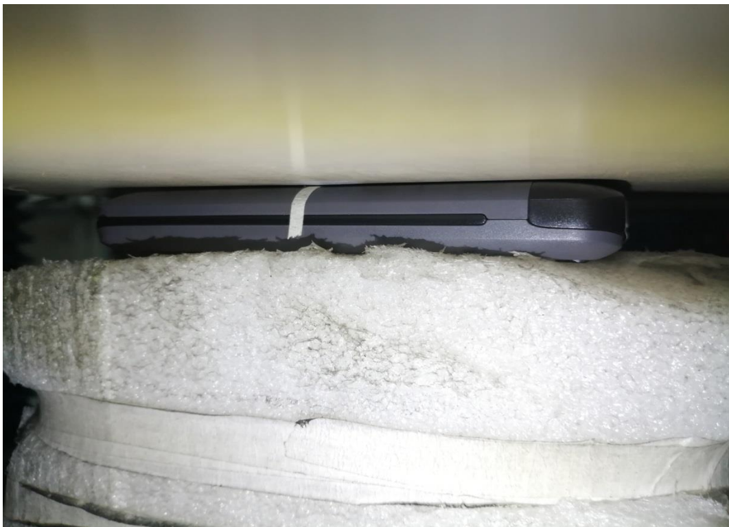
DUT without device holder (DUT direct contact with the phantom)
