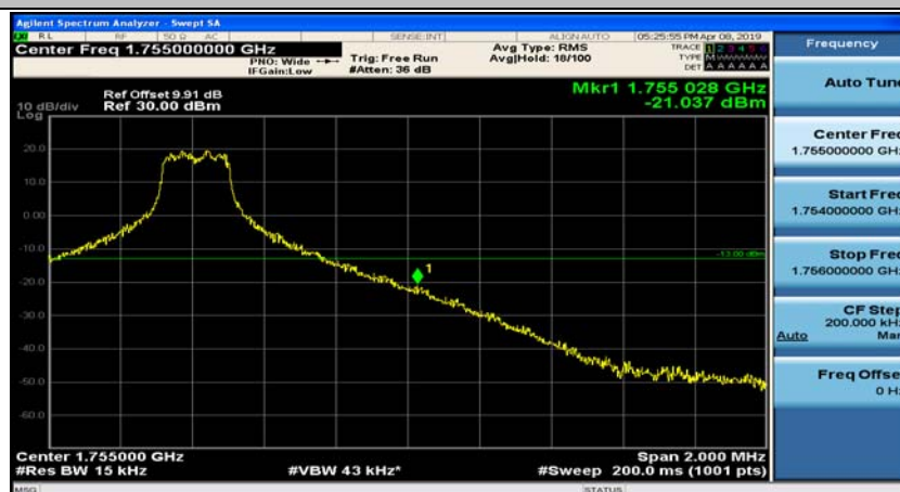
Channel Bandwidth: 10 MHz_HCH_16QAM_25RB#0
