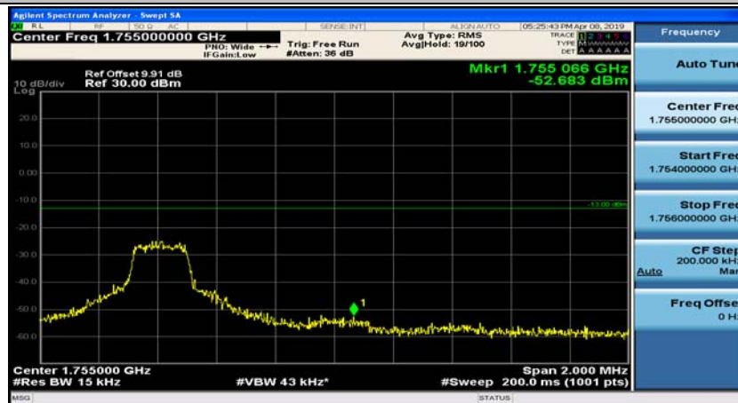
Channel Bandwidth: 10 MHz_HCH_16QAM_1RB#24
