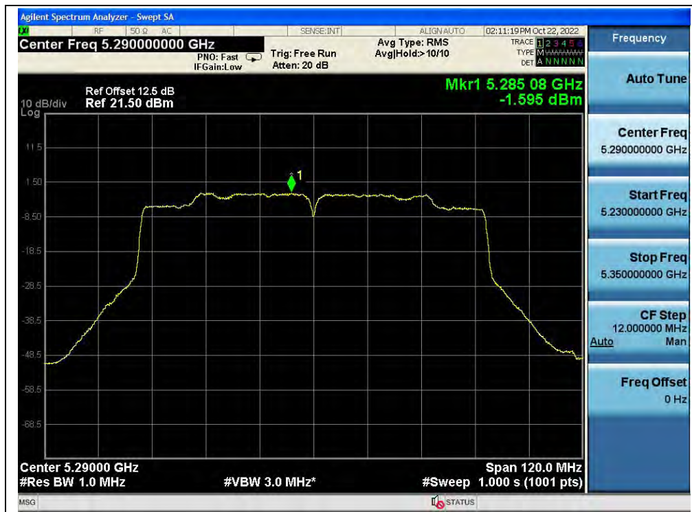
(Channel 58, 5290MHz, 802.11ac (VHT80), ANT0)
