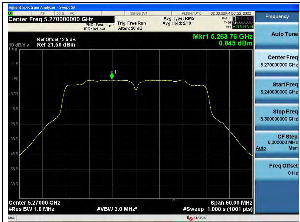
(Channel 54, 5270MHz, 802.11ac (VHT40), ANT0)
