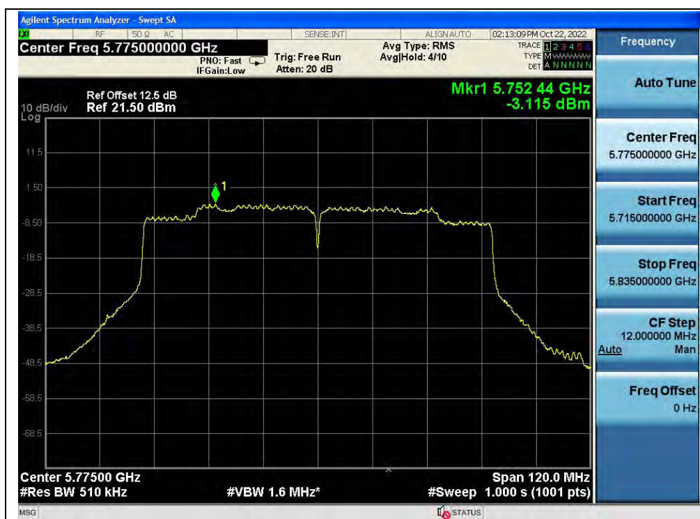
(Channel 155, 5775MHz, 802.11ac (VHT80), ANT0)
