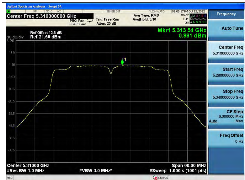
(Channel 62, 5310MHz, 802.11ac (VHT40), ANT0)
