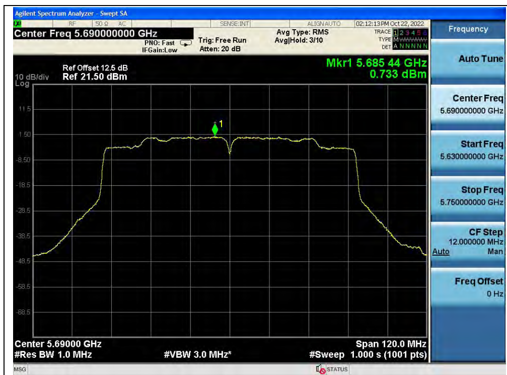
(Channel 138, 5690MHz, 802.11ac (VHT80), ANT0)
