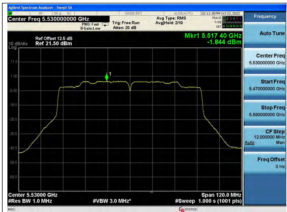
(Channel 106, 5530MHz, 802.11ac (VHT80), ANT0)
