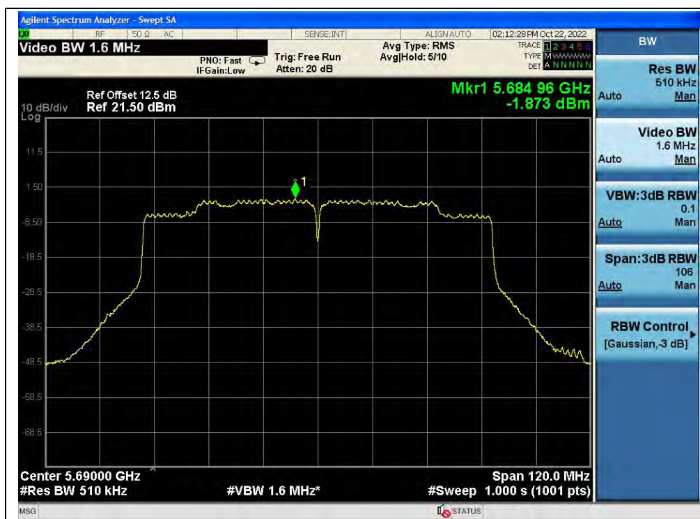
(Channel 138, 5690MHz, 802.11ac (VHT80), ANT0)
