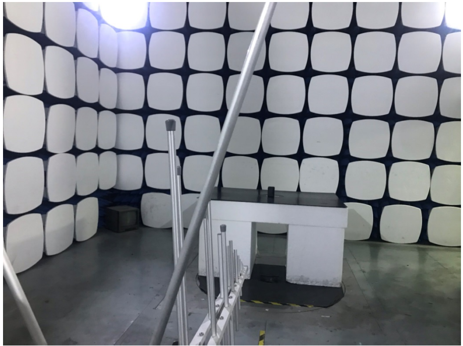
Radiation Emission Test Setup (30MHz to 1GHz)
