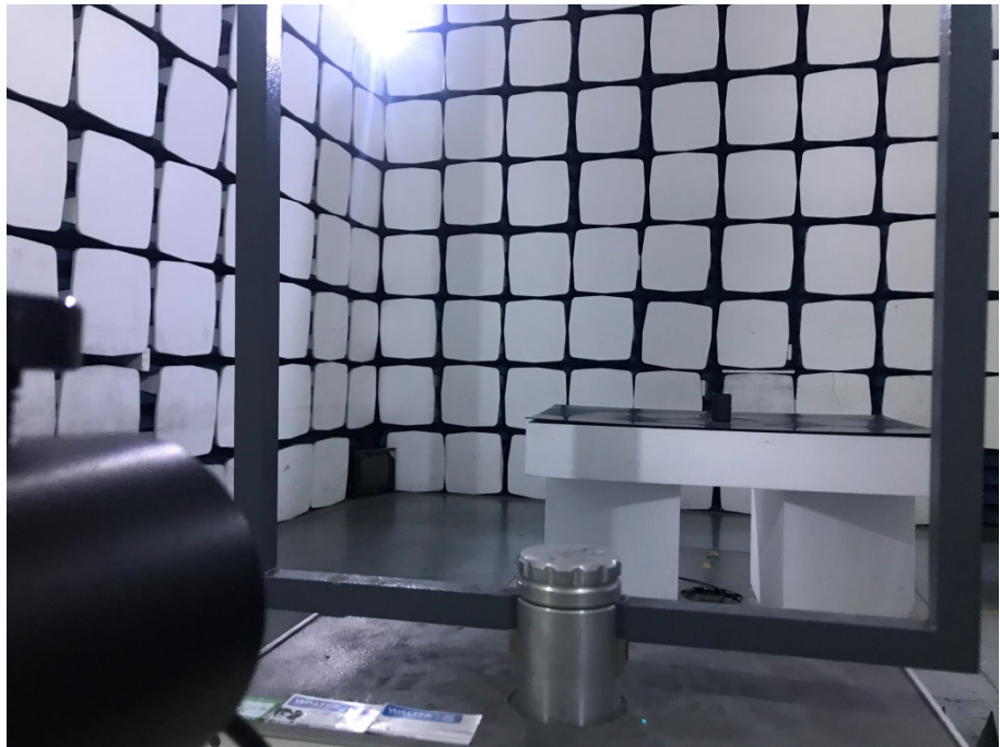
Radiation Emission Test Setup (Below 30MHz)
