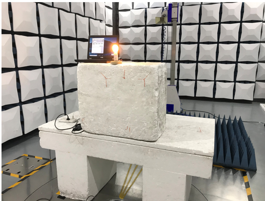
Radiated Disturbances Rear Side (Above 1GHz)
