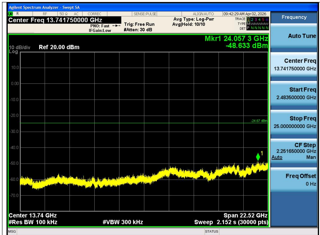
Test_Graph_LE1M_ANT1_2402_1Mbps_Higher Band Emissions
