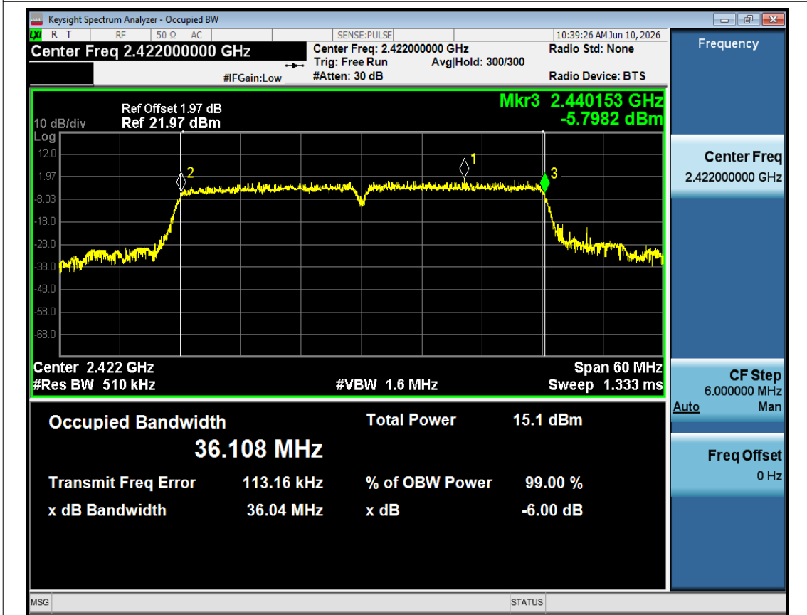
-6dB Bandwidth NVNT n40 2422MHz Ant1
