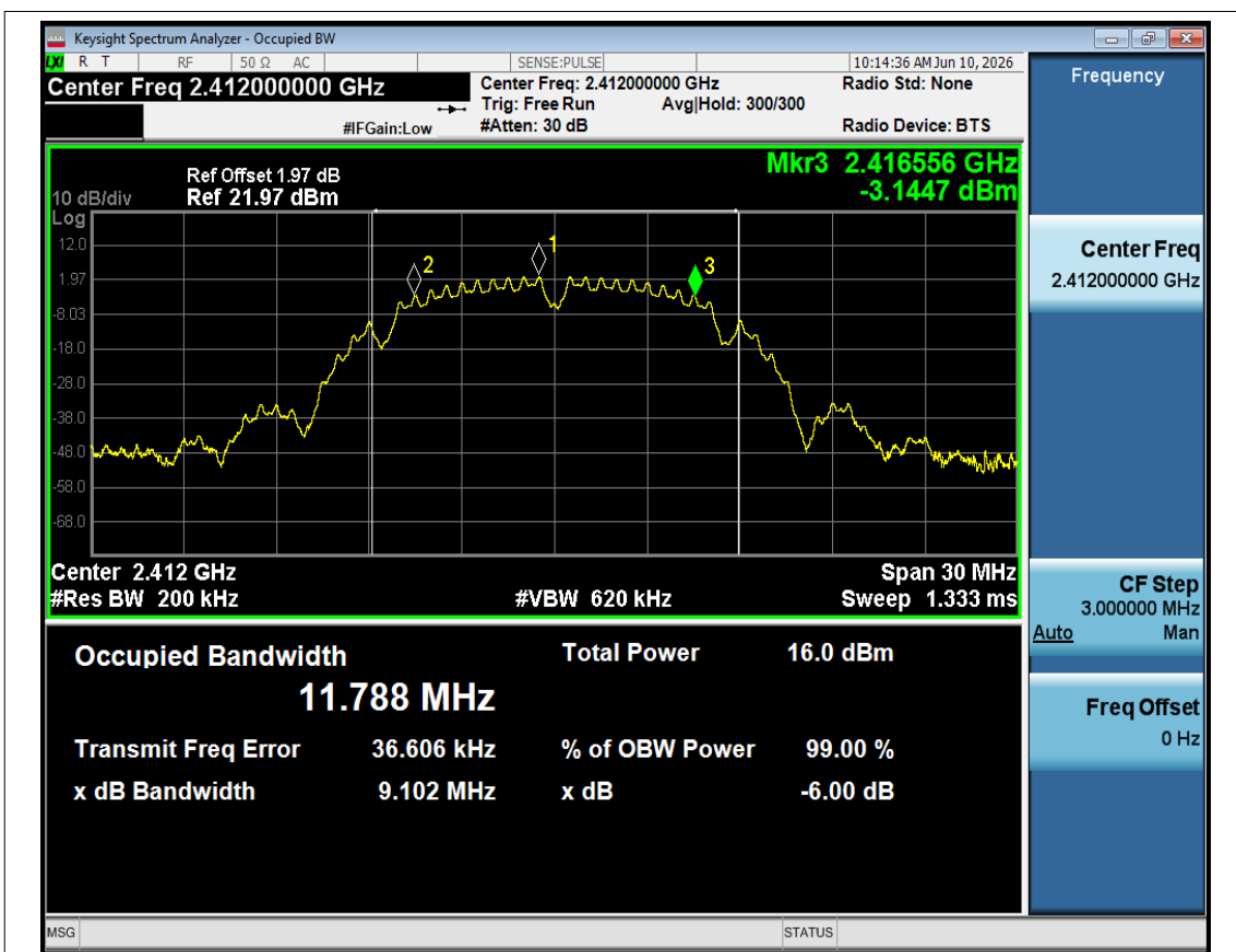
-6dB Bandwidth NVNT b 2412MHz Ant1
