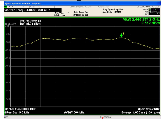
In-Band Reference Level BLE 1M_Channel 19
