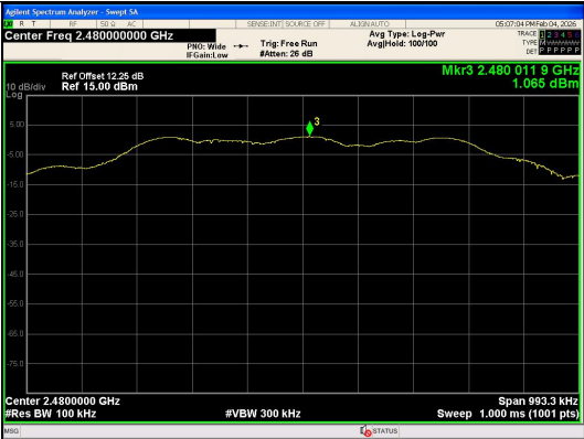
In-Band Reference Level BLE 1M_Channel 39
