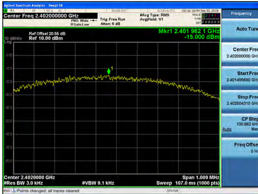
Power Spectral Density (Low-CH 0)
