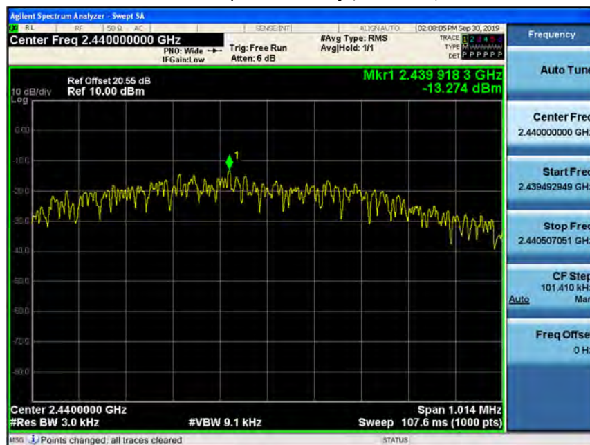
Power Spectral Density (Mid-CH 19)
