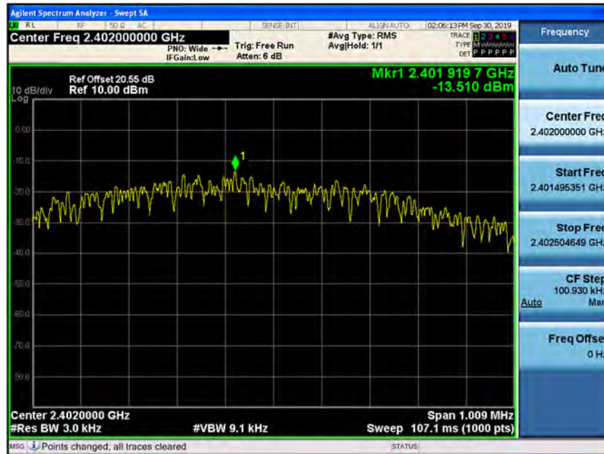
Power Spectral Density (Low-CH 0)
