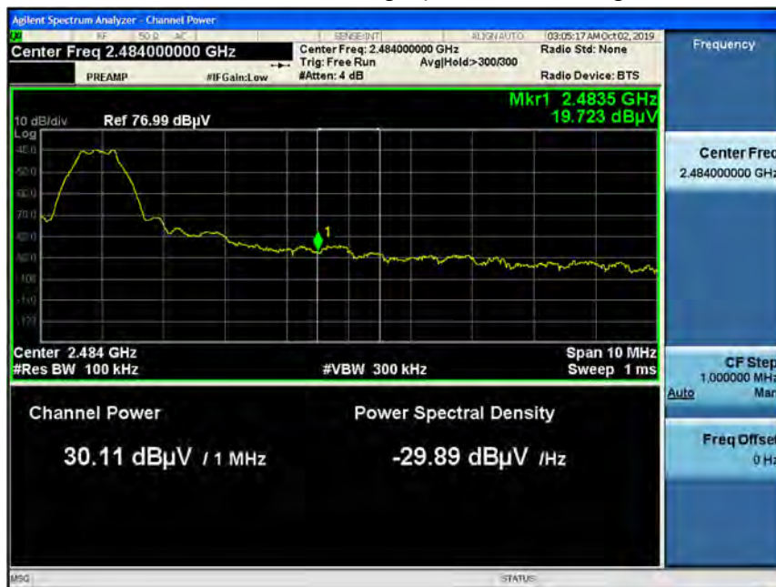
Radiated Restricted Band Edges plot – Peak Reading (Ch.39)
