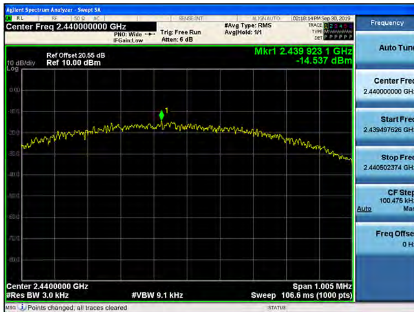
Power Spectral Density (Mid-CH 19)
